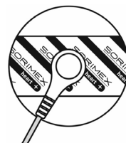
Fig. 1. Way of leadwire and electrode connection
