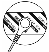
Fig. 1. Way of leadwire and electrode connection
